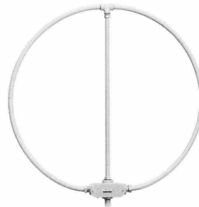
Fig. 10. Weatherproof antenna used with Comparator System.
